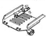
4. Position the angle adjustor bar at the desired angle between the location bars.
