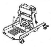
Slip the safety clamp plate/s back into position and tighten the safety bar knobs securely.
