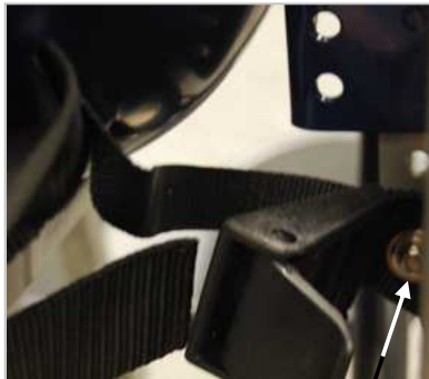
Lower straps bolted to frame
