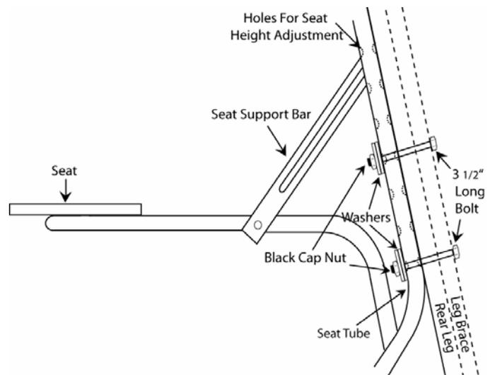
Figure 3: Seat Installation
