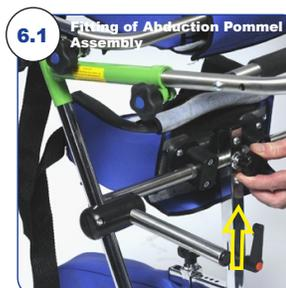
If an abduction pommel is fitted to the Trekker or Tiny Trekker it will be necessary to locate this into position using the plunger hand-wheel which will locate into the hole on the hip rail. The hand-wheel can then be tightened to secure the abduction pommel.
