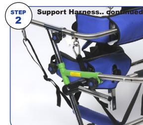
Re-insert the chest rail into the frame. Repeat the procedure with the two remaining harness brackets. Align the brackets and tighten the white hand-wheels. You can now clip on the support harness.
